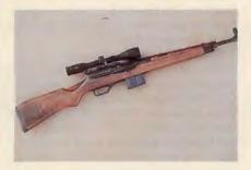
The HK SL6/7 weapons are actually a carbine-length version of the HK 630/770/940-series sporting rifles. "SL" presumably stands for Self-Loading (Selbstlade). The numbers "6" and "7" are rough approximations, in millimeters, of the overall cartridge length the action will accept. The SL6 is chambered for the 5.56mm NATO (.223 Rem.) cartridge. SOF's test rifle is an SL7, which is chambered for my favorite GPMG and sniping-rifle round, the 7.62x51mm NATO (.308 Win.) cartridge.
